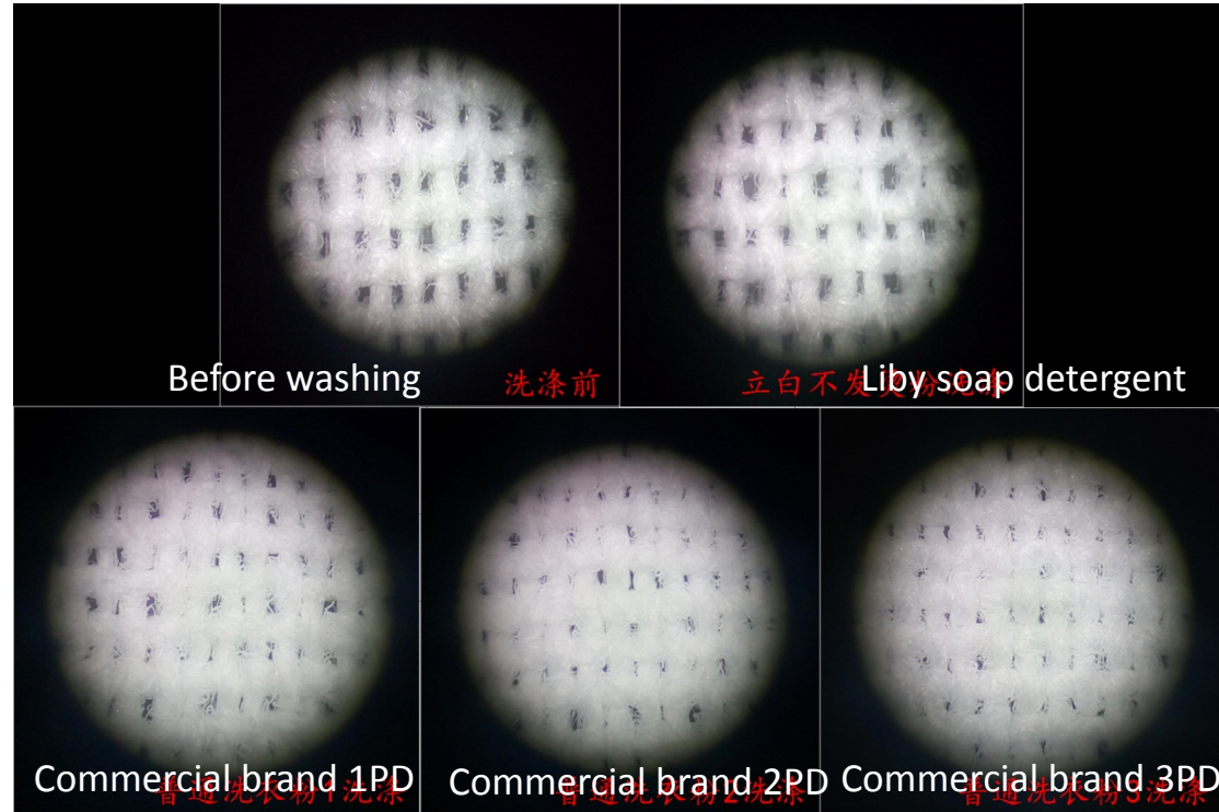
Microscope image of fabric after washing for 20 cycles.
